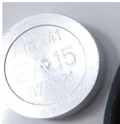
Figure 9.1: Solid alpha source typically used in laboratories with a diameter of 2 cm.
